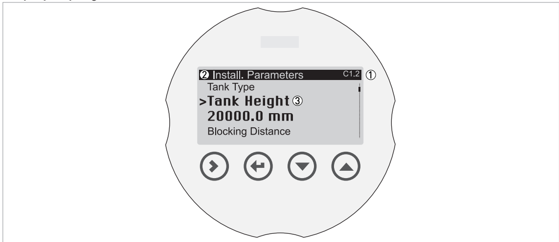
Figure 5-2: Display screen layout in program mode
