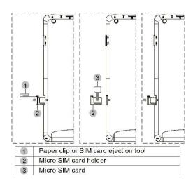
$\textbf{Note} \hbox{: The SIM card can't be recognized if it is inserted when the tablet is powered on.} \\$
