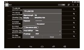
5. Tap the IP settings box to select Static, complete the IP address, Gateway, Network prefix length, DNS1 and DNS2 (the settings in the figure below are for reference only), and then tap Connect to complete the network connection.
