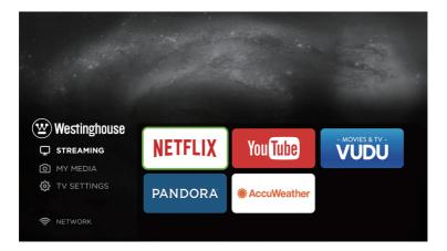
Press MENU to display the main interface, then use the Arrow buttons to highlight STREAMING and press OK to confirm. Use the Arrow buttons to cycle among different options and select desired apps to enter.
