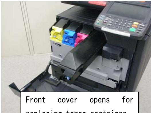
Front cover opens for replacing toner container.
