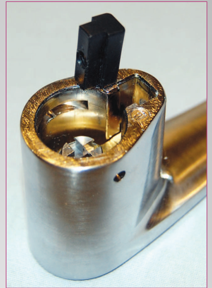
10. Insert the lock cylinder into the lever.
