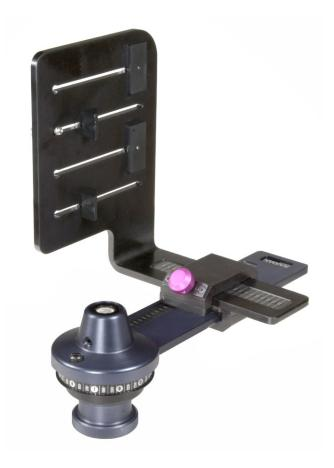
The left-right adjustment to center your lens over the pivot point is accomplished by loosening the purple knob and sliding the camera bracket in and out of the slider. Be sure to tighten the knob to lock the bracket in place.
