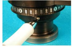
Removing Indexing Rings
