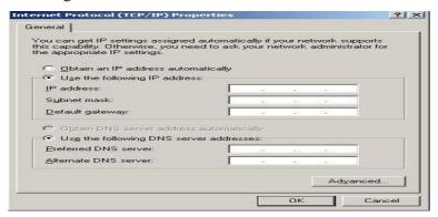
> C Fill the IP address blank, example as below:
