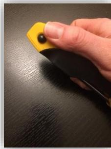
WHP1 – Press the probe release and extend the sensing probe 90° or 180° until it locks in place.
