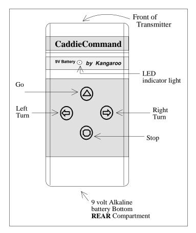
The position of the transmitter is important during signal transmission. In order to achieve maximum range, hold the transmitter with the control buttons on top and the back of the transmitter toward the ground. Point the front of the transmitter toward the motorcaddie. The transmitter will operate if held otherwise, but the overall operating range will be decreased. The range will also be affected if there are obstacles between you and the motorcaddie such as trees, buildings, cars, etc.
