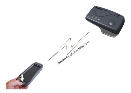
The typical reading range is up to 3m (10feet) and depends on these parameters:
