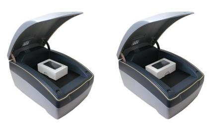
Figure 7 Incorrect positions of packed OBUs
