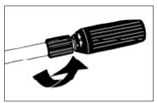
Step 2 The wand must be set in the low pressure (-) position to apply detergents.
