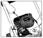
Step 8 Pull the starter handle. If the engine fails to start after 3 pulls squeeze the trigger gun to release pressure, and repeat step 8.
