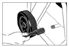
Step 4 Connect high pressure hose to high pressure outlet.
