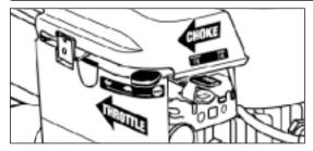
Step 7 Slide the throttle control to the fast position. Move the ckoke lever to the "CHOKE" position (only if the engine is cool). After starting, move the choke to "RUN".
