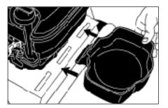
**Step 1** Slide the detergent tray into one of the slots of your choice. Secure the tray to the frame by fastening the screw.
