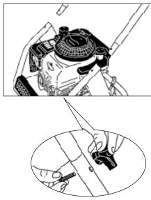
Step 2 Align the holes of the accessory rack to the handle and fasten the four screws.
