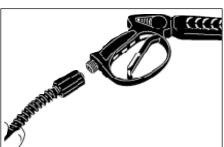
Step 5 Attach high pressure hose to trigger gun.
