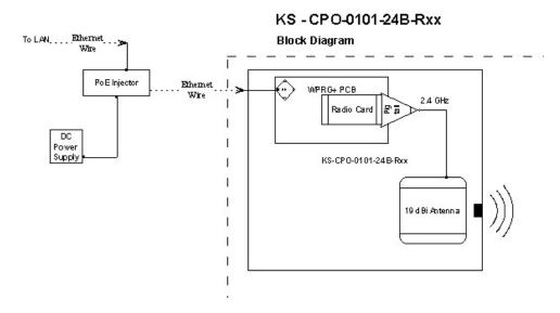
KarlNet CPE Outdoor products operate with the included Power over Ethernet (PoE) injector. When planning an installation using PoE, it is important to consider the power requirements of the CPE Outdoor system and the length of the Ethernet cable that will carry the power. The table shown below specifies the injector specifications required to deliver power to the CPE Outdoor device over various lengths of Ethernet Cable.
