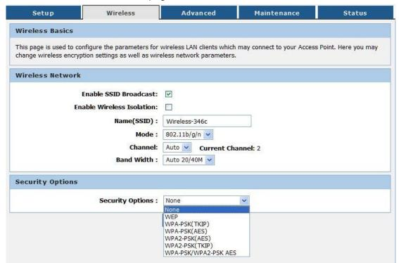
Name (SSID): Also called the SSID. Enter a value of up to 32 characters. The same name must be assigned to all wireless devices in your network.
