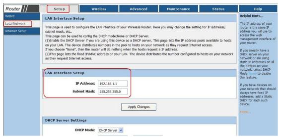
**IP Address**:Enter the IP address of your Router or reset it in dotted-decimal notation (factory default: 192.168.0.1).
