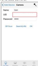
3. There are 2 ways to enter the camera's UID quickly, by scanning the QR code on the camera and search the cameras in LAN. Click **Scan** to initiate the scan and click **Search** to search the cameras in LAN.
