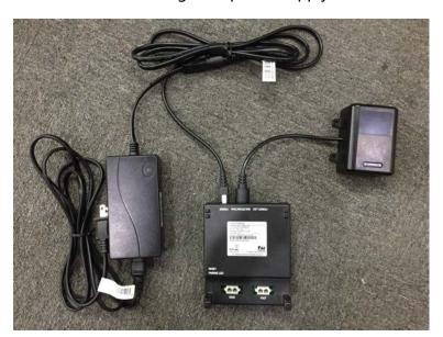
Double click reset key, the LED will be on. Long press the back button of the remote, the LED will be flash. When two LEDs are off, the connection of the remote and the control box is completed.
