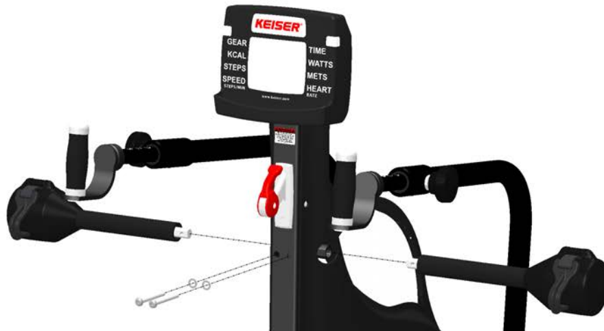
Figure 4. Left and Right Recoiler Installation
