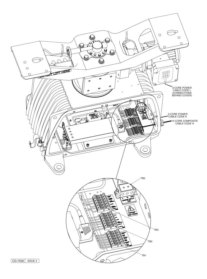
Figure 7 - Transceiver (DTX-A3): Cableform Routing
