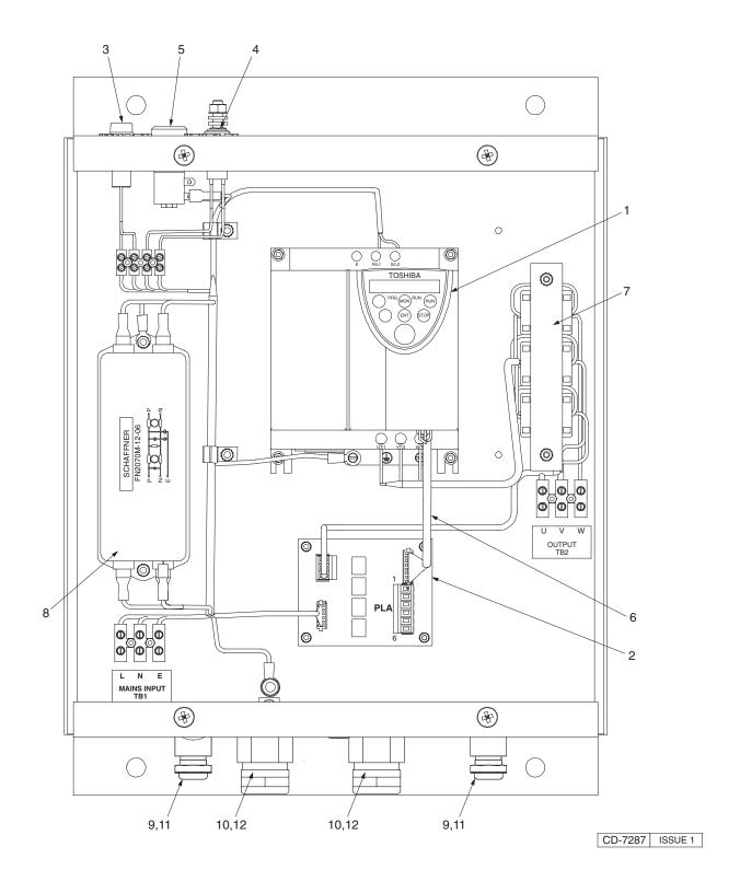
Figure 2 - Drive Control Unit (GTX-A24): Main Assemblies
