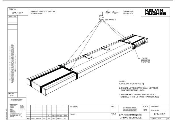
Figure 4 - Suggested Antenna Lifting Arrangement
