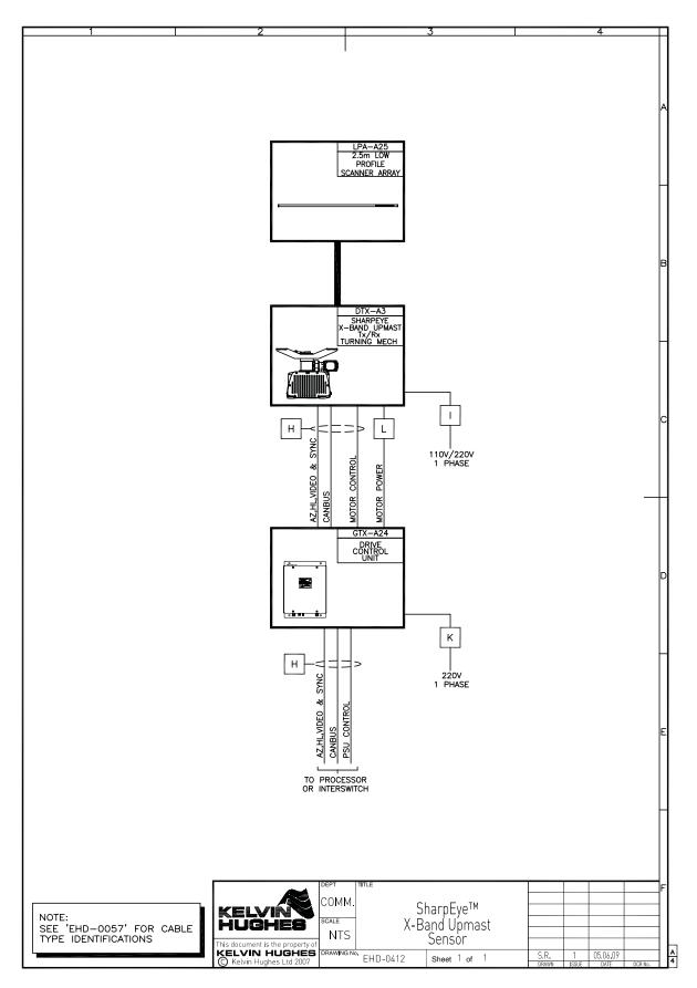
Figure 2 - *SharpEye*<sup>™</sup> Transceiver: Typical Configuration
