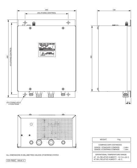
**Figure 5 - Drive Control Unit (GTX-A24): Installation Dimensions**
