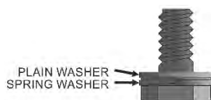
Example of bolt and washer arrangement
