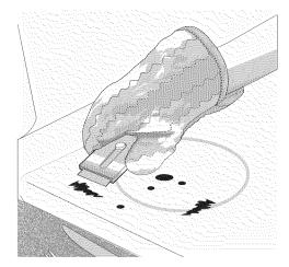
Figure 37: Using razor blade to remove burned on matter
