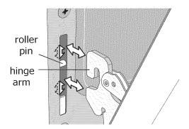
Figure 45: Location of hinge arm and roller pin
