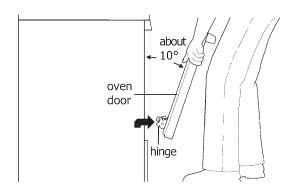
Figure 44: Holding door for removal
