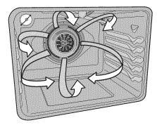
Figure 21: Air circulation in the convection function
