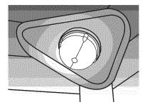
Figure 38: Replacing the oven light
