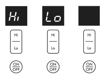
Figure 10: Highest setting, Lowest setting, and OFF.
