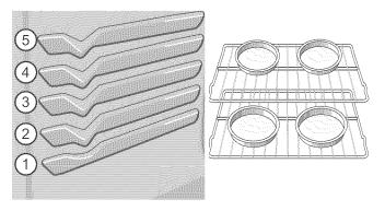
Figure 22: Convection rack positions and pan spacing
