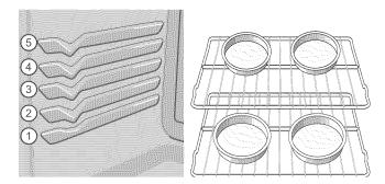
Figure 20: Rack positions and pan spacing recommendations
