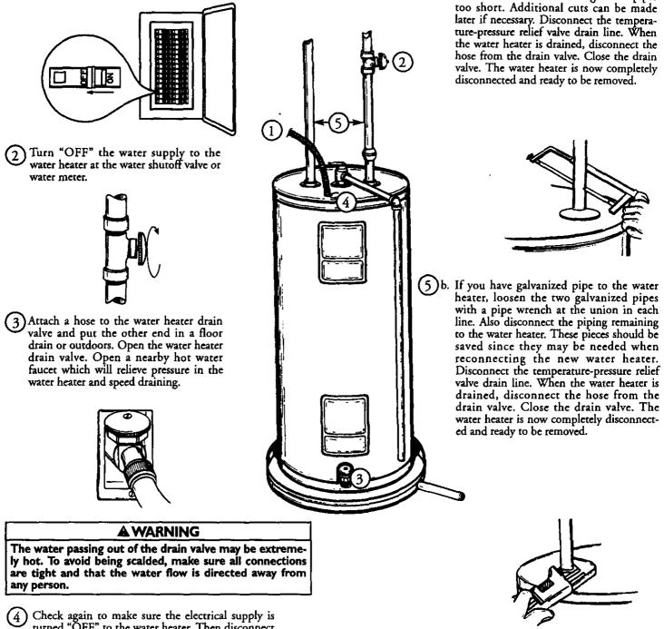
turned "OFF" to the water heater. Then disconnect the electrical supply connection from the water heater junction box.
