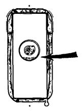
12. The adjustment dial has a "D" shaped opening that matches a "D" shaped shaft on the thermostat. Align the opening in the dial to the shaft and gently push the dial onto the shaft.
