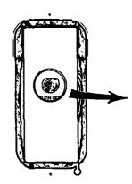
7. Lift out the tab as shown to unclip the terminal cover from the thermostat. The terminal cover can now be removed from the thermostat.
