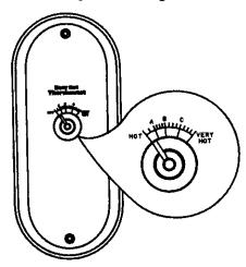
LOWER THERMOSTAT ADJUSTABLE THROUGH LOWER ACCESS PANEL
