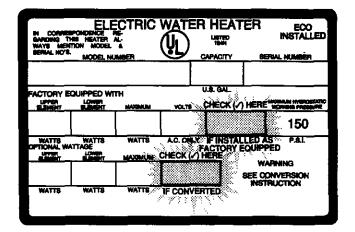
NOTE: Whether or not the element conversion is made the model rating plate must be marked. Using a hard point ink pen, check the appropriate block within the model rating plate, which is located adjacent to the lower access panel.
