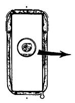
5. Lower Element: Lift out the tab as shown to unclip the terminal cover from the thermostat. The terminal cover can now be removed from the thermostat.
