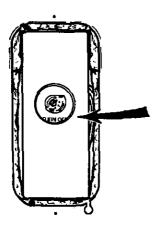
19. The adjustment dial has a "D" shaped opening that matches a "D" shaped shaft on the thermostat. Align the opening in the dial to the shaft and gently push the dial onto the shaft.
