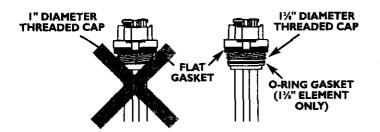
NOTE: These instructions are written for element cleaning and element replacement for the lower element. If it is necessary to clean or replace the upper element, then repeat these instructions.
