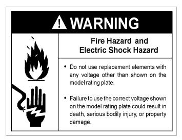
Replacement elements must (1) be the same voltage and (2) no greater wattage than listed on the model rating plate affixed to the water heater.
