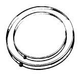
METAL DRAIN PANS AVAILABLE IN 20" DIAMETER FOR WATER **HEATERS HAVING A DIAMETER 18"** OR LESS AND IN 24" DIAMETER FOR WATER HEATERS HAVING A DIAMETER OF 22" OR LESS.
