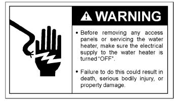
Before beginning, turn "OFF" the electric power supply to the water heater. After the power has been turned off, open a nearby hot water faucet until the water is no longer hot.
