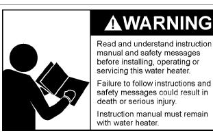
Read this manual first. Then before checking the water heater make sure the electric supply has been turned "OFF", and never turn the electric supply "on" before the tank is completely full of water.
