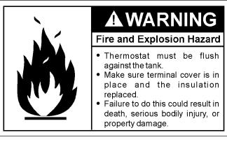
Make sure the thermostat is flush against the tank, the terminal cover is in place, and the insulation is replaced. Failure to do so can result in DEATH, SERIOUS BODILY INJURY, OR PROPERTY DAMAGE.
