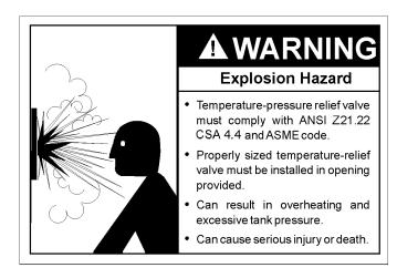
This heater is provided with a properly certified combination temperature - pressure relief valve by the manufacturer.
