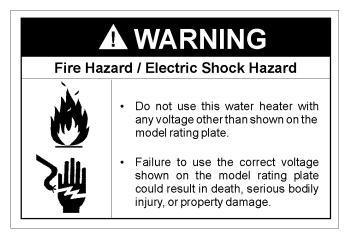
Before making the conversion to 5500 watts, make sure that the (1) power supply is 240 volts, (2) the wiring is 10 gauge AWG @ Type TW, 60°C or equivalent, and (3) the circuit breakers or fusing are capable of 30 amp loading. Also, the installation must conform with this manual, local codes and electric utility rules. Failure to comply can result in DEATH, SERIOUS BODILY INJURY, OR PROPERTY DAMAGE.
