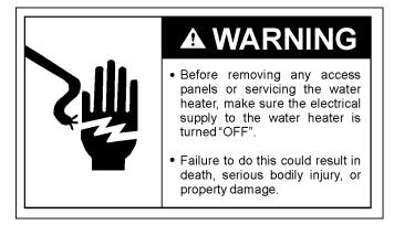
Before beginning, turn "OFF" the electric power supply to the water heater. After the power has been turned off, open a nearby hot water faucet until the water is no longer hot.
