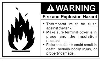
Make sure the thermostat is flush against the tank, the terminal cover is in place, and the insulation is replaced. Failure to do so can result in DEATH, SERIOUS BODILY INJURY, OR PROPERTY DAMAGE.
