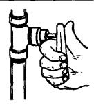
2 Turn "OFF" the water to the water heater. Some installations require that the water be turned off to the entire house.
