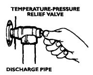
Failure to install and maintain a new properly listed temperature-pressure relief valve will release the manufacturer from any claim which might result from excessive temperature or pressure.
