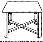
WATER HEATER STAND 24"x24"x18" FOR USE WITH WATER HEATERS INSTALLED IN RESIDENTIAL GARAGES HAVING A DIAMETER 24" OR LESS AND A RATED CAPACITY 75 GALLONS OR LESS
