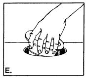
Now, push the strainer up through the sink hole and remove it.
