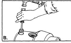
Tap the end of the screwdriver with a hammer until the molded plug pops out. Make sure you take the loose plug out of your disposer.
