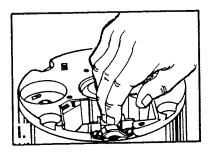
Finally, place the connected wires back in the compartment. Replace electrical plate.
