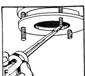
Loosen screws and remove old mounting ring and back-up ring. You may need a harmmer to loosen assembly parts.
