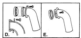
In D. install the discharge tube gasket onto the discharge tube. Gasket must be installed as shown to assure a leak-proof installation. In E. install discharge tube gasket into disposer discharge outlet. Gasket will be held in place by the discharge tube flange.
