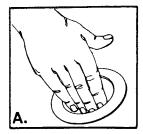
First, check inside the disposer grinding chamber to remove any objects or dirt that might have dropped in.
