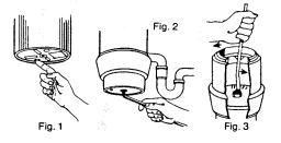
A pry bar or tool should be inserted through the sink opening into the disposer. The end then must be placed alongside the grinding protrusion near the outside edge of the grinding disc. Be sure to place the pry tool on the proper side of the protrusion so when pressure is applied the grinding disc will move in the proper direction to unjam the disposer. (see Fig. 3). Do not drop or hammer on pry bar.
