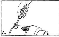
Lay the disposer on its side and put the tip of your screwdriver into the dishwasher drain hole opening at an angle.
