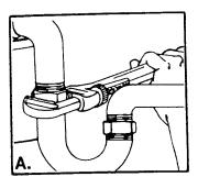
Use a pipe wrench to disconnect the drain line where it attaches to the disposer discharge tube.
