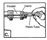
Insert one end of the plastic tube into the coupler and fasten with % inch clamp.
