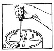
Once the disposer is off, turn it upside down and remove the electrical plate.
