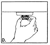
Loosen the nut until you can spin it off by hand.
