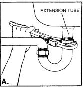
Use a pipe wrench to loosen the nut at the top of the drain trap.
