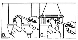
Turn the disposer around to attach the discharge tube. Some models use a rubber washer that must be assembled to the discharge tube before putting the metal flange over the discharge tube, see 'D'. Secure metal flange using the edge tab on the flange and screw. On other models, put the rubber washer in the discharge tube opening. Slip the metal flange over the discharge tube. Using the screw(s) provided, attach the flange to disposer, see 'E'.
