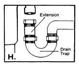
TUBE TOO SHORT? If the discharge tube doesn't reach your drain trap outlet, measure the difference. Then buy a drain extension tube
