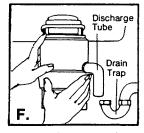
Turn the disposer so that the discharge tube lines up with your drain trap. Slip the drain trap over the discharge tube.
