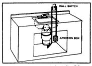
It will be necessary to install a 20 amp. wall switch above the countertop and a junction box under the sink as illustrated.
