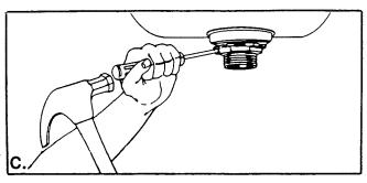
Now, remove the large nut at the base of the sink strainer by placing the tip of your screwdriver on the edge of the nut. (There are usually ridges to hold your screwdriver.) Then strike the head of the screwdriver with a hammer in a counterclockwise direction.
