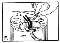
Work the cable from the on-off switch through the connector so that the leads are in the electrical wiring area in the disposer base.
