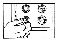
First, remove the fuse or turn off the circuit breaker on the circuit you plan to use for your disposer. Use a separate 15 or 20 amp., 115 volt circuit for the disposer.
