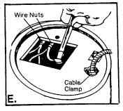
Now, use a screwdriver to remove ground wire. Remove the wire nuts from the power wires. Separate the disposer power wires from the cable wires. Loosen the screw(s) on the cable clamp and remove the cable from the disposer.
