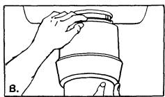
Then, while holding the disposer in place, turn mounting ring with the lugs to the right until all three ears are engaged on the mounting assembly. The disposer will now hange by itself. You will lock this ring later, after the plumbing connections are made.
