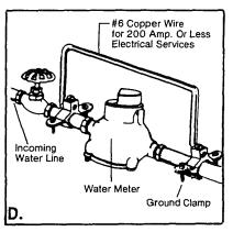
**WARNING:** IF NOT PROPERLY GROUNDED, a hazard of electrical shock may exist. DO NOT reconnect electrical power at main service panel until proper ground is installed. For your safety, DO NOT ground to a gas supply pipe.
