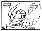
First, remove the mounting assembly from the lower mounting ring. Holding the mounting assembly with one hand, insert your wrenchette or screwdriver into one of the lugs of the lower mounting ring and turn it to the left (counterclockwise) with your other
