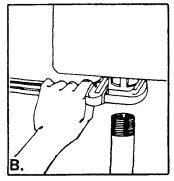
Next, remove the nut at the top of the sink strainer and remove the extension tube.
