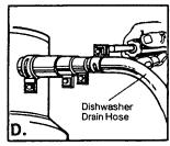
Slip the remaining clamp (the one you pruchased) over the dishwasher drain hose and back two or three inches. Now, slip the drain hose over the plastic tube, slide the clamp into place and tighten.
