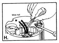
Install the cable connector. Then loosen the connector screw(s). Work the cable from the on-off switch through the connector so that the leads are in the electrical wiring area in the disposer base.
