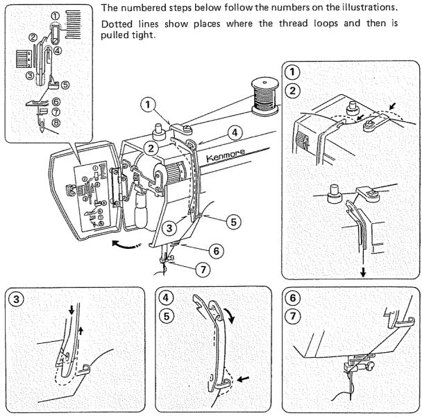
Raise thread take-up lever to its highest position by turning hand wheel toward you. Raise presser foot lever. Place spool on spool pin as shown, with thread coming from the back of the spool.
