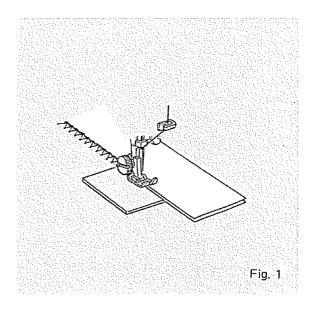
This stitch can be used for sewing a seam with an overcast finish. It is used for seams of 3/8" to 1/4". The seam is formed and finished in one operation. It must be used when you are making swimwear, ski pants and other garments that require stretch.
