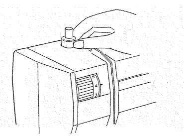
Push down the outer ring of the pressure regulator. This will release the pressure on the presser foot. (See above)
