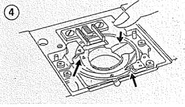
4. Insert the shuttle into the shuttle race making sure to line up red arrows as illustrated in Fig. 4. The bobbin should be fully seated.
