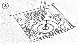
Using a small brush, remove the lint that accumulates in and around the feed dogs and shuttle area. And put a drop of oil to the point indicated by arrow.
