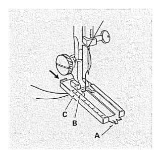
1. Carefully mark the buttonhole length on your garment. Place the fabric with the buttonhole marked under the buttonhole foot. Pull the guide foot (A) all the way forward so that the index mark (B) is aligned with the graduation (C), with thread to rear. (The markings on the left side of foot will help you in making all your buttonholes the same size. Graduations act as reference mark.)
