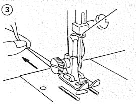
3. Pull both threads under and to the back of the presser foot, leaving 3 to 4 inches of thread clear.
