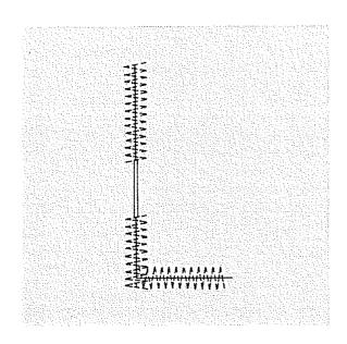
To repair a straight or three-cornered tear, position the tear under the needle in such a way that the stitching catches both sides of the tear. When mending a three-cornered tear, stitch from each end to the center. It is well to use a piece of fabric under the tear for reinforcement.
