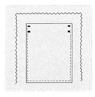
This stitch is similar to a very short satin stitch and is used to reinforce points of strain such as corners of pockets and straps on lingerie.
