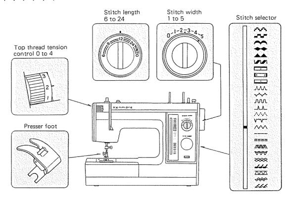
This type of stitching greatly expands the use of your machine. This is the feature that enables you to overcast seams, applique and sew on buttons. Simply use the settings indicated in the illustration for the simple zigzag. Follow directions given in the following pages for more specific uses.
