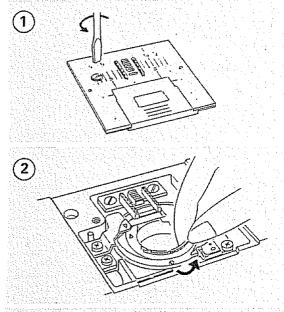
To insure the best possible operation of your machine, it is necessary to keep the essential parts clean at all times. Using a small brush, remove the lint that accumulates in the shuttle area and around the feed dogs.
