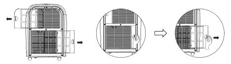
Cleaning: Wash the air filter by immersing it in lukewarm water and a mild detergent. Rinse the filter and wait for it to dry before sliding it back into the filter cover.
