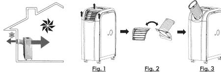
The cold air emitted from unit must exit the room through the exhaust hose connected to the window kit.
