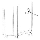
NOTE: In DEHUMIDIFY, ventilator fan speed is preset to maximize efficient operation. You will not be able to adjust the fan speed. You may also allow the water to drain by opening the lower drain outlet and placing the unit directly over a shallow pan. Do not leave the unit unattended in case the pan fills and needs to be emptied.
