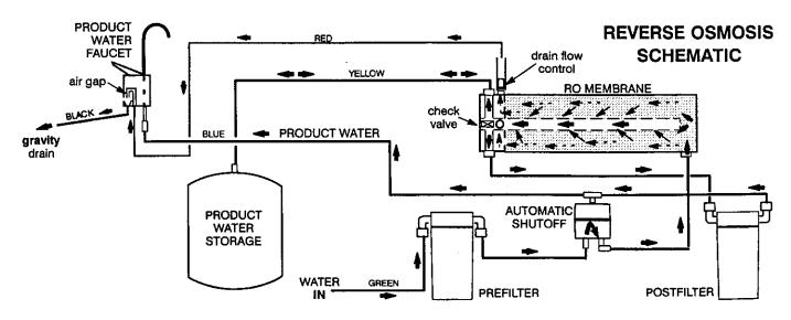
To keep your reverse osmosis system operating and making high quality water, you must make sure supply water is always within the limits shown in the specifications. Good supply water helps to assure longer life from the RO membrane cartridge, prefilter and postfilter cartridges. However, each of these will wear out in time and need replacement.
