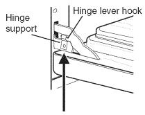
Lock engaged for door removal Figure 1
