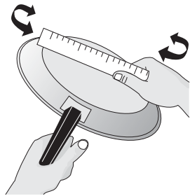
Figure 2: Check pan for flat bottom using ruler
