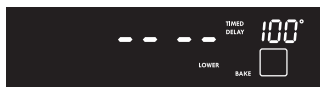
Figure 20: Dashes appear showing oven control ready for cook time to be entered
