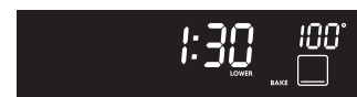
Figure 18: Display shows time of day and the actual oven temperature above the oven icon
