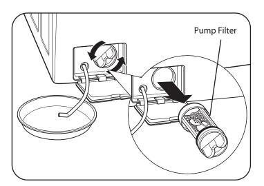
4 Twist the pump filter counterclockwise to remove. Remove any lint and foreign objects from the pump filter. Insert the pump filter back into the opening and twist clockwise to secure. Be sure to close the drain pump filter access panel.
