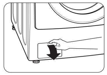
Open the drain pump filter access panel.
