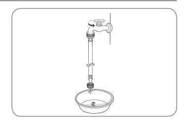
3. Always run a gallon or two of water through each inlet hose to flush dirt, scale and other debris out of the water lines. Doing so will help prevent future problems with clogged filter screens, and will also allow you to verify which water line is hot and which is cold.
