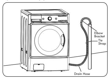
Install the end of the drain hose into the elbow bracket. Do not extend the drain hose more than 4 inches past the end of the elbow bracket. Use a tie strap to secure the drain hose in place.
