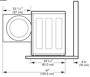
To ensure sufficient clearance for water lines and airflow, allow minimum clearances of at least 1 in. (2.5 cm) at the sides and 4 in. (10 cm) behind the unit. Be sure to allow for wall, door, or floor moldings that may increase the required clearances.
