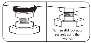
3. Once the washer is level from side to side and front to back, use the adjusting wrench to tighten all four lock nuts securely to prevent the legs from getting out of adjustment during operation. Make sure that all four leveling feet are in firm contact with the floor.
