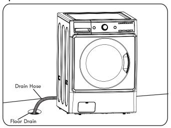
Insert the end of the drain hose into the floor drain. If possible, secure the hose to prevent it from moving or coming out of the drain.
