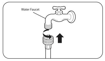
2. Connect the water supply hoses to the HOT and COLD water faucets tightly by hand and then tighten another ½ turn with pliers.
