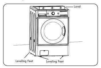
1. Position the washer in its final location, taking special care not to pinch, strain, or crush the water and drain lines. Place a level across the top of the washer.
