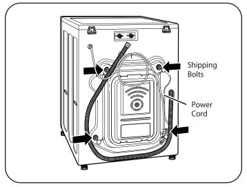
1. Starting with the bottom two shipping bolts, use the wrench (included) to fully loosen all four shipping bolts by turning them counterclockwise.
