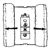
7. Lift out the tab as shown to unclip the terminal cover from the thermostat. The terminal cover can now be removed from the thermostat.
