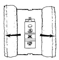
5. Lower Element: Lift out the tab as shown to unclip the terminal cover from the thermostat. The terminal cover can now be removed from the thermostat.
