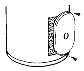
14. Complete wiring to the water heater, or if completed, turn "ON" electric power to the water heater <u>after</u> filling the tank with water.
