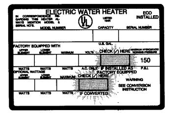
NOTE: Whether or not the element conversion is made the model rating plate must be marked. Using a hard point ink pen, check the appropriate block within the model rating plate, which is located adjacent to the lower access panel.
