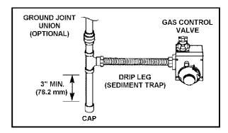
FIGURE 19. GAS PIPING WITH FLEXIBLE CONNECTOR.
