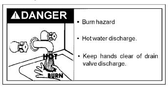
4 Attach a hose to the water heater drain valve and put the other end in a floor drain or outdoors. Open the water heater drain valve. Open a nearby hot water faucet which will relieve pressure in the water heater and speed draining. The water passing out of the drain valve may be extremely hot. To avoid being scalded, make sure all connections are tight and that the water flow is directed away from any person, see Figures 2 and 5.
