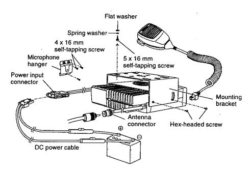
\* The above diagram shows the TK-780 series/ TK-880 series transceiver. The antenna connector of the TK-980 and TK-981 transceivers is different.
