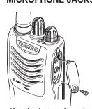
If you are not using a speaker/ microphone, install the cover over the speaker/ microphone jacks using the supplied 3 x 6 mm screw.
