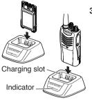
Slide a battery pack or a transceiver equipped with a battery pack into the charging slot of the charger.
