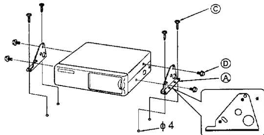
**Vertical installation / Installation verticale / Instalación vertical**
