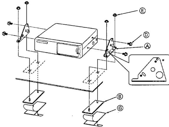
\* Attach the brackets with the screws inserted in the blackened holes. (Do the same for the left side also.)
