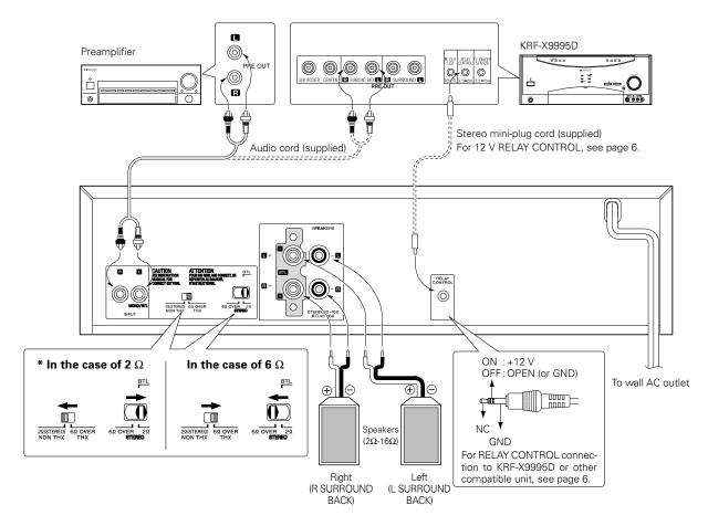
\* If you connect more than one pair of speakers to the KMF-X9000, move the  $2\Omega$  (STEREO)/ $6\Omega$  OVER (THX) switch to the  $2\Omega$  (STEREO) position. The amplifier's performance is not THX®-certified when the switch is set in the  $2\Omega$  (STEREO) position.
