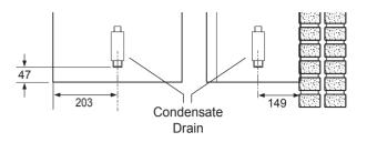
This appliance is fitted with a siphonic 75mm condensate trap system that requires filling before operating the appliance for the first time or after maintenance.
