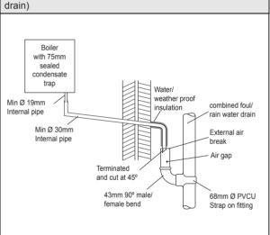
Figure 6 - Connection of Condensate Drainage Pipe Upstream of a Sink, Basin, Bath or Shower Waste Trap to External Drain, Gulley or Ranwater Hopper Boiler with 75mm sealed condensate Visible air break trap at plug hole Water/ weather proof Min Ø 19mm insulation Internal pipe Sink, basin, bath or Minimum 30mm grate shower with integral internal pipe overflow and 75mm trap Below ( > 25 | 45° pipe termination
