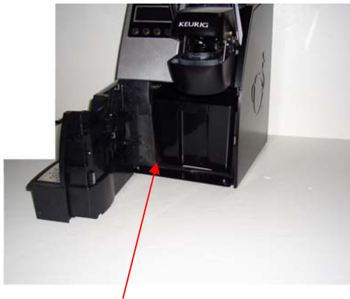
DOOR FULLY OPEN WITH K-CUP BIN VISIBLE
