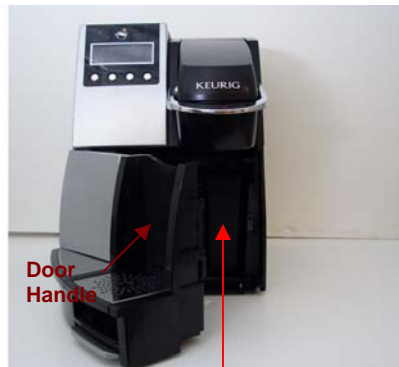
BREWER DOOR IS HINGED, ALLOWING ACCESS TO K-CUP BIN
