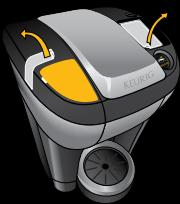
**A** Remove all adhesive tape and labels. Lift Handle and remove shipping disc. Lower Handle. Plug into grounded outlet.
