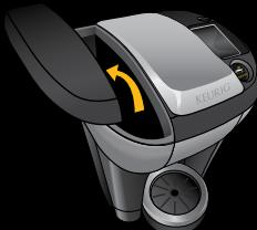
**B** Carefully remove Water Reservoir Lid. Remove Water Reservoir by lifting up and away from the brewer.
