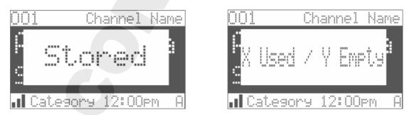
2. By holding down the MEMO button for 3 seconds, the stored memory information (one at a time) is displayed on the LCD screen in page format. Use the Channel knob to scroll through the 30-page listing and view the information. This function allows you to recall information regarding the Artist/Song Title for your own personal review. To return to the default tuning mode press and hold the MEMO button for 3 seconds.
