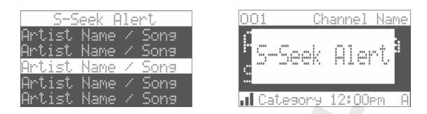
No stored match alert is provided for the currently selected stream. To ensure that no duplicate entries are stored in memory, the receiver will check the stored input data to ensure the information about to be stored is not already in memory.
