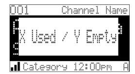
2. By holding down the MEMO button for 3 seconds, the stored memory information (one at a time) is displayed on the LCD screen in page format. Use the Channel knob to scroll through the 30-page listing and view the information. This function allows you to recall information regarding the Artist/Song Title for your own personal review. To return to the default tuning mode press and hold the MEMO button for 3 seconds.
