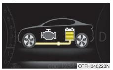
Hybrid battery is being charged by regenerative braking. (Wheel  $\rightarrow$  Battery)
