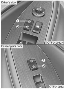
If the key is in the ignition switch (or if the smart key is in the vehicle) and any front door is opened, the doors will not lock when the "Lock" position (1) of the central door lock switch is pressed. (if equipped)
