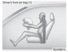
The air bag modules are located both in the center of the steering wheel and in the front passenger's panel above the glove box. When the SRSCM detects a sufficiently severe impact to the front of the vehicle, it will automatically deploy
