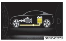
Electric and Engine power are used to move the vehicle. (Battery & Engine → Wheel)
