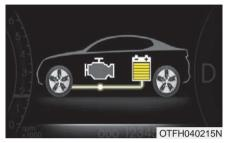
Motor power is used to move the vehicle. (Battery  $\rightarrow$  Wheel)
