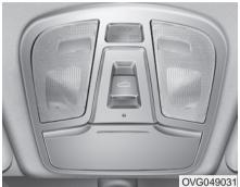
OVG049031 If your vehicle is equipped with a sunroof, you can slide or tilt your sunroof with the sunroof control lever located on the overbead console
