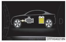
Engine power is used to move the vehicle. (Engine  $\rightarrow$  Wheel)
