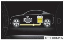
Hybrid battery is being charged by regenerative braking. (Wheel → Battery)
