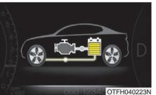
The vehicle is being slowed by engine compression and regenerative braking. The hybrid battery is being charged by regenerative braking. (Engine  $\rightarrow$  Battery  $\rightarrow$  Wheel)
