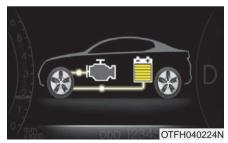
The engine friction is used to vehicle brake system and the regenerative brake charges the hybrid battery. (Wheel  $\rightarrow$  Engine & Battery)
