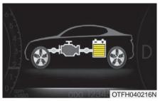
Engine is both driving the vehicle and charging the hybrid battery. (Engine  $\rightarrow$  Wheel & Battery)
