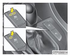
*Climate control seat (if equipped)* The climate control seat is provided to cool or warm the seat during hot or cold weather by blowing air through small vent holes on the surface of the seat and seatback. While the engine is running, push the rear portion of the switch to cool the seat, and push the front portion of the switch to warm the seat.
