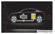
Electric power is used to move the vehicle. (Battery  $\rightarrow$  Wheel)
