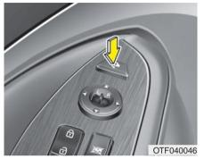
Folding the outside rearview mirror **Electric Type (if equipped)** To fold the outside rearview mirror. depress the button.
