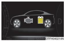
The mode means the vehicle stop. (No energy flow)
