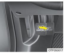
*Releasing the parking brake* Foot type
