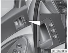
A driver position memory system is provided to store and recall the driver seat position with a simple button operation. By saving the desired position into the system memory, different drivers can reposition the driver seat based upon their driving preference. If the battery is disconnected, the position memory will be lost and the driving position should be
