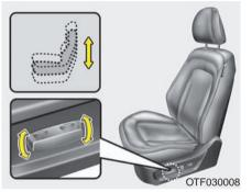
Seat height (for driver's seat) Pull the front portion of the control switch up to raise or down to lower the front part of the seat cushion. Pull the rear portion of the control switch up to raise or down to lower the rear part of the seat cushion. Release the switch once the seat reaches the desired position.
