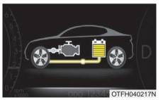
Motor and Engine power are used to move the vehicle. (Battery & Energy  $\rightarrow$  Wheel)
