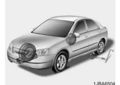
To prevent vehicle movement while changing a tire, always set the parking brake fully, and always block the wheel diagonally opposite the wheel being changed.
