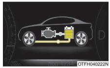
The engine and regenerative brake system charges the hybrid battery. (Engine & Wheel  $\rightarrow$  Battery)
