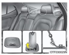
Securing a child restraint seat with tether anchorage system Child restraint hook holders are located on the package tray.
