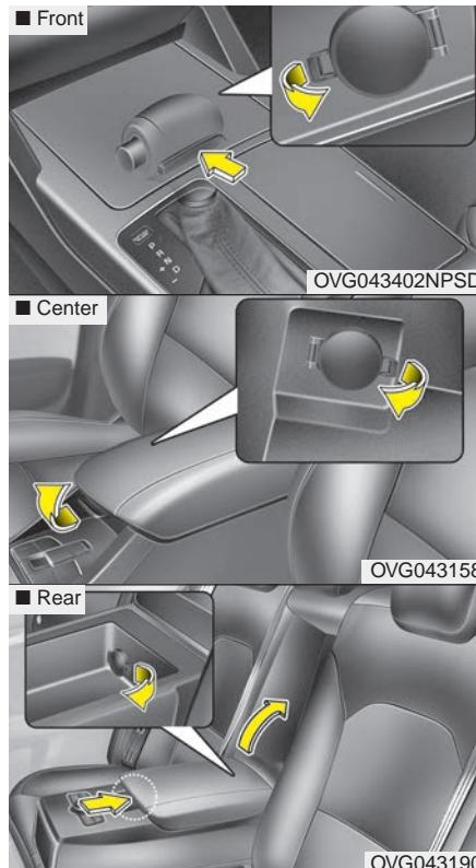
The power outlet is designed to provide power for mobile telephones or other devices designed to operate with vehicle electrical systems. The devices should draw less than 10 amps with the engine running.
