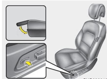
Press the front portion of the switch to raise the cushion extension, or the rear portion of the switch to lower it. Release the switch once the cushion extension reaches the desired position.
