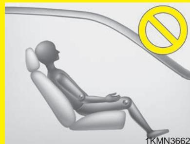
The driver must advise the passenger to keep the seatback in an upright position whenever the vehicle is in motion. If a seat is reclined during an accident, the restraint system's ability to restrain will be greatly reduced.
