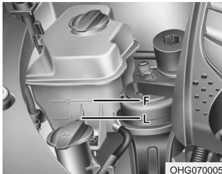
If the coolant level is low, add enough distilled (deionized) water. Bring the level to F (MAX), but do not overfill. If frequent coolant addition is required, see an authorized Kia Premium dealer for a cooling system inspection.
