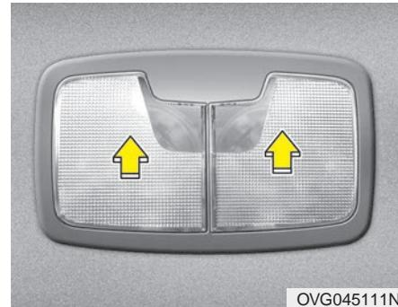
Press the lens to turn the room lamp on and off.
