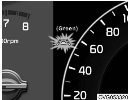
To operate the LDWS, press the switch with the engine start/stop button in the ON position. The indicator illuminates on the cluster. To cancel the LDWS, press the switch again.
