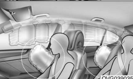
Your vehicle is equipped with a side air bag in each front and outboard rear seat.
