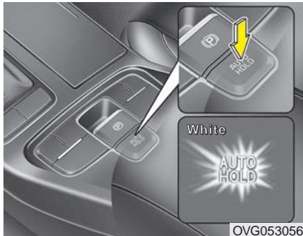
1. Depress the brake pedal and then press the Auto Hold button. The white AUTO HOLD indicator will come on and the system will be in the standby position. The driver's door, engine hood and trunk closed and the driver's seat belt must be fastened before EPB will work.
