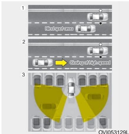
The Blind Spot Detection System (BSD) uses a radar sensor to alert the driver.
