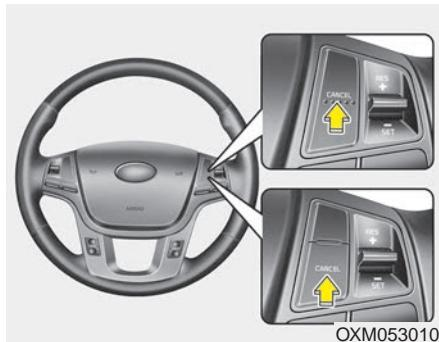
Each of these actions will cancel cruise control operation (the *SET* indicator light in the instrument cluster will go off), but it will not turn the system off. If you wish to resume cruise control operation, move the lever up (to *RES+*). You will return to your previously preset speed.
