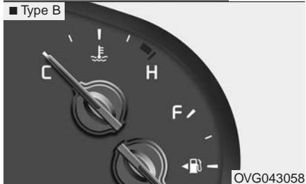
This gauge indicates the temperature of the engine coolant when the ignition switch or Engine Start/Stop button is ON.
