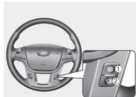
The LCD display modes can be changed by using the control buttons on the steering wheel.
