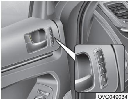
A driver position memory system is provided to store and recall the driver seat, outside rearview mirror and steering wheel positions\* with a simple button operation. By saving the desired positions into the system memory, different drivers can reposition the driver seat, outside rearview mirror and steering wheel based upon their driving preference. If the battery is disconnected, the position memory will be lost and the driving positions should be restored in the system.
