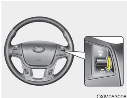
3. Lever must be moved down (to SET-) prior to setting any desired speed. The SET indicator light in the instrument cluster will illuminate. Release the accelerator at the same time. The desired speed will automatically be maintained.
