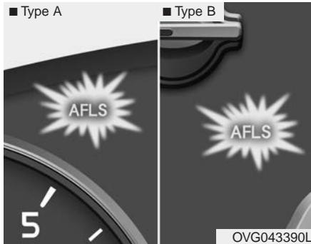
If the AFLS malfunction indicator comes on, the AFLS is not working properly. Drive to the nearest safe location and restart the engine. If the indicator is still on, have the system checked by an authorized Kia Premium dealer.
