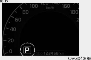
This indicator displays which automatic transaxle shift lever is selected.
