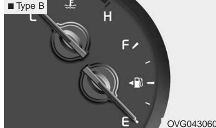
This gauge indicates the approximate amount of fuel remaining in the fuel tank.
