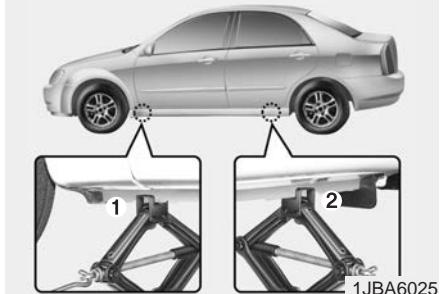
7. Place the jack at the front (1) or rear (2) jacking position closest to the tire you are changing. Place the jack at the designated locations under the frame.
