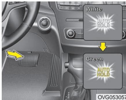
2. When you stop the vehicle completely by depressing the brake pedal, the AUTO HOLD indicator changes from white to green.
