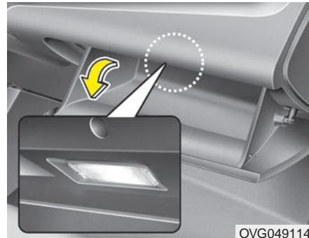
The trunk room lamp comes on when the trunk is opened. The trunk light comes on only with the trunk lid open. To prevent battery discharge, close the trunk lid securely after accessing the trunk.
