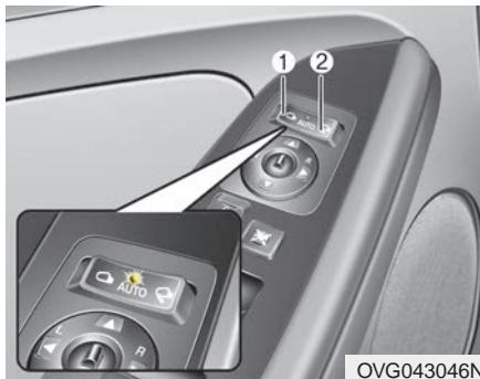
The outside rearview mirror can be folded or unfolded by pressing the switch as below.
