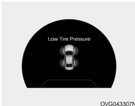
When the tire pressure monitoring system warning indicators are illuminated and warning message displayed on the cluster LCD display, one or more of your tires is significantly under-inflated. The low tire pressure position telltale light will indicate which tire is significantly under-inflated by illuminating the corresponding position light.
