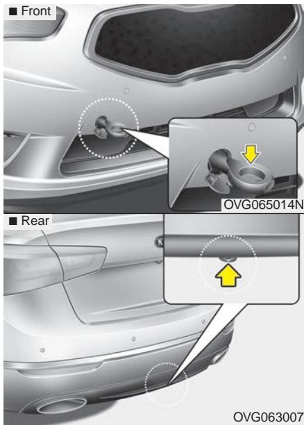
If towing service is not available in an emergency, your vehicle may be temporarily towed using a cable or chain secured to the emergency towing hook under the rear of the vehicle. Use extreme caution when towing the vehicle. A driver must be in the vehicle to steer it and operate the brakes.
