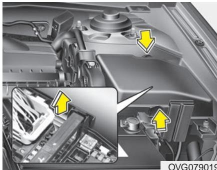
3. Pull the suspected fuse straight out. Use the fuse puller provided in the engine compartment fuse panel.
