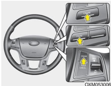
1. Push the CRUISE button on the steering wheel to turn the system on. The CRUISE indicator light in the instrument cluster will illuminate.
