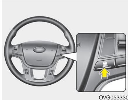
This system allows you to set and maintain the distance from the vehicle ahead of you without pressing the accelerator or brake pedal.
