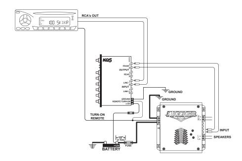
When only one source unit is used it doesn't matter which set of input jacks are used. Just make sure the input selector switch on the KQ5 front panel is in the correct position(in for Line 2 input, out for Line 1 input). Likewise, if only one set of RCA cables are run to your amplifier(s), make sure the Fader Control is turned to the direction that gives you output to the jacks being used (clockwise for rear, counter-clockwise for front).
