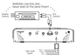
The use of twisted pair interconnects is recommended for all installations to minimize noise. When routing these cables through the automobile, try to keep them away from factory wiring harnesses and other power wiring. If you need to cross any of this wiring do so at a 90 degree angle to reduce the possibility for noise problems.
