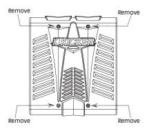
With the shroud removed, you now have access to the four mounting holes in the mounting feet and all wiring connections. Drill 4 holes using a 7/64" drill bit and use the supplied #8 screws to mount the amplifier.
