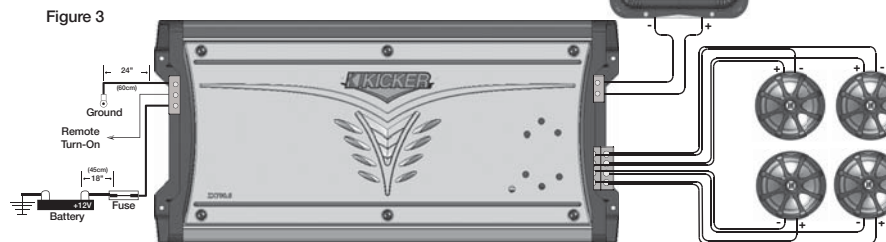
(ZX550.3) Two Channel Operation with Subwoofer
