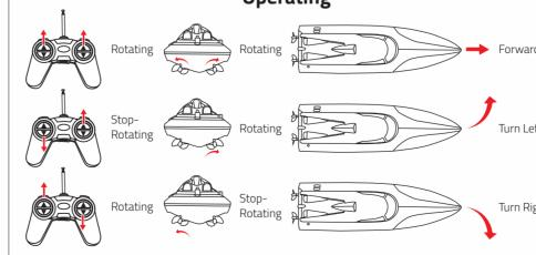
When both levers are pushed upward simultaneously, the boat will go forward. When the right lever is pushed upward and the left lever is pushed down, the boat will turn left. When the left lever is pushed forward and the right lever is pushed down the boat will turn right.
