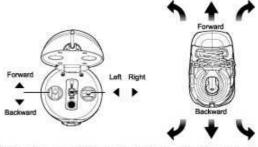
Drive the sneaker over the ball. Conveyor belt inside the sneaker will scoop the ball up to the top white sneaker is moving.
